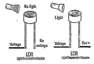
Figure 1. Light dependent Resistor
