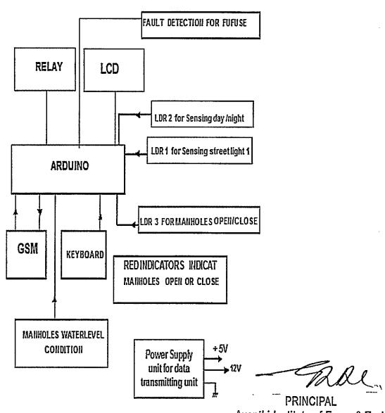
Figure 3. Block Diagram of street light control with manhole monitoring Avanthi Institute of Engg. & Tech Guadapally (V), Abdullapurmet (Mdl), R.R. Dist.
